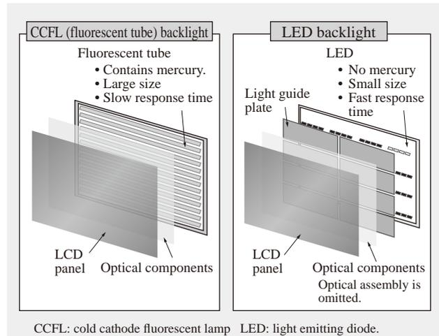
Fig. 4—Outline of CCFL and LED Backlight Structure. Whereas a CCFL backlight operates continuously regardless of the input picture signal, an S-LED backlight consumes less power because its intensity is controlled area by area based on the input picture signal.
