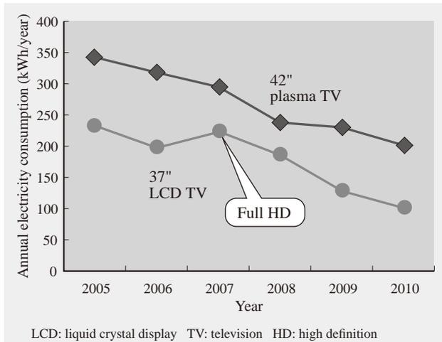
Fig. 3—Trend in Annual Electricity Consumption of Flat-panel Televisions due to Energy Efficiency Improvement. The figures 2009 and 2010 are obtained using the new measurement procedure stipulated in the April 2010 revisions to the Act on the Rational Use of Energy criteria (standards of judgment for manufacturers/importers with regard to the improvement of the performance for the TV sets).
