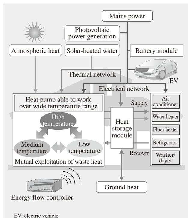
Fig. 6—Example Configuration of Future Home Energy System. To expand the use of renewable energy, the system features a heat pump able to work over a wide temperature range and unforced refrigerant circulation, all of which is operated by an integrated energy control system.
