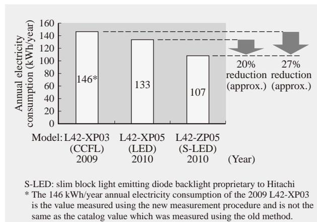
Fig. 5—Difference in Annual Electricity Consumption of 42" LCD Televisions with Different Types of Backlight (Measured Using Measurement Procedure Stipulated in April 2010 Revision of Act on the Rational Use of Energy Criteria). The annual electricity consumption for a television is calculated in accordance with the Act on the Rational Use of Energy criteria based on an average household viewing time of 4.5 h/d and average standby time of 19.5 h/d.
