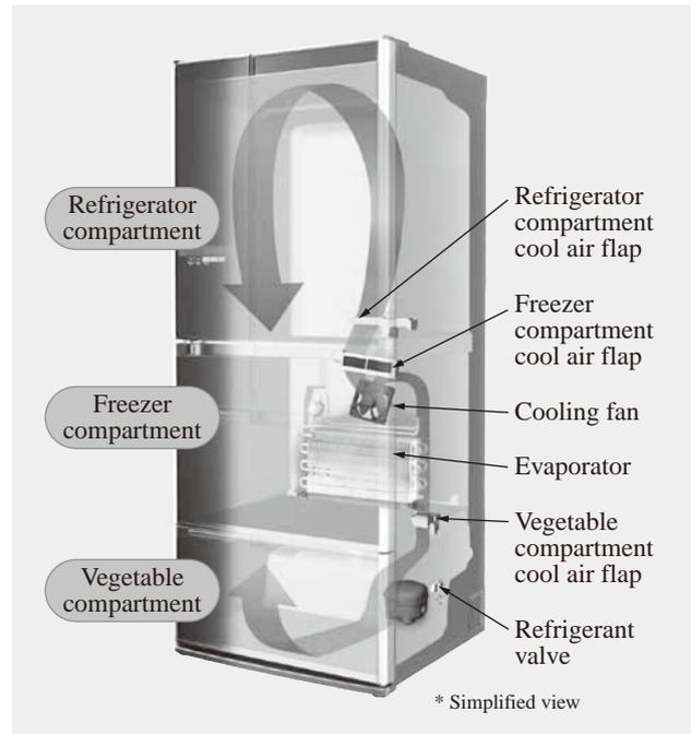
Fig. 1—Overview of Frost Recycling Technology.
