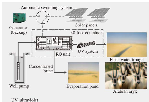
Fig. 3—Flow Chart of Solar RO System.
