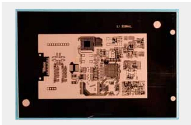
Fig. 8—Prototype Printed Circuit Board Made from Epoxy Resin with Lignin as its Main Raw Material.
