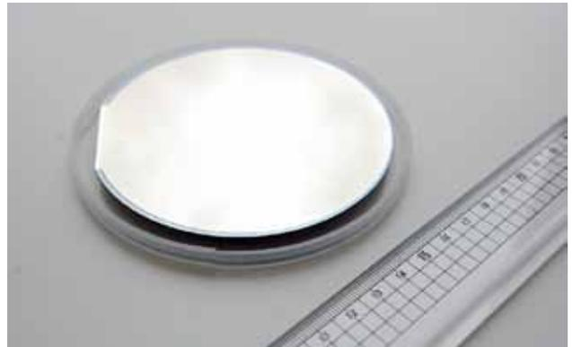
Fig. 7—(K, Na) NbO<sub>3</sub> Piezoelectric Thin Film Formed on 4-inch Silicon Wafer.
