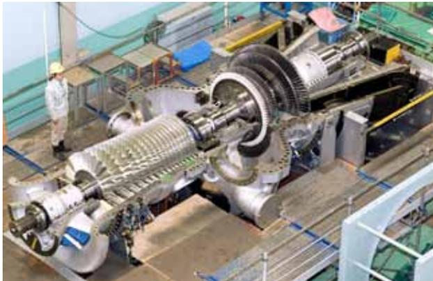
Fig. 8—Cutaway Photograph of 40-MW-class AHAT Gas Turbine.
