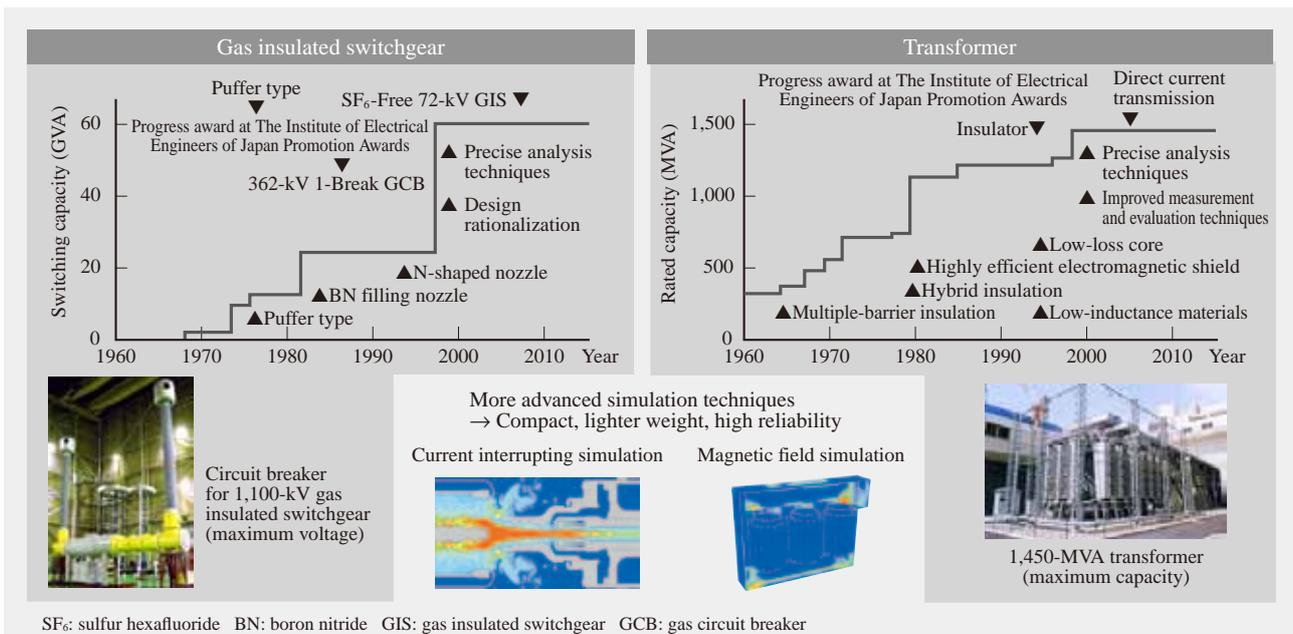
Fig. 12—Development of Electrical Substation Equipment. Hitachi is achieving better efficiency, smaller size, and higher capacity through the use of numerical simulation for optimization and to elucidate the phenomena involved.
