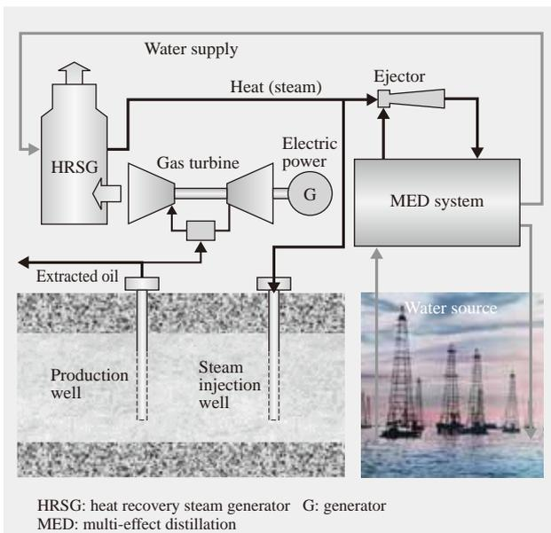
Fig. 10—Trigeneration System Producing Electric Power, Heat, and Water. The waste heat from the gas turbine is recovered and used to produce purified water.
