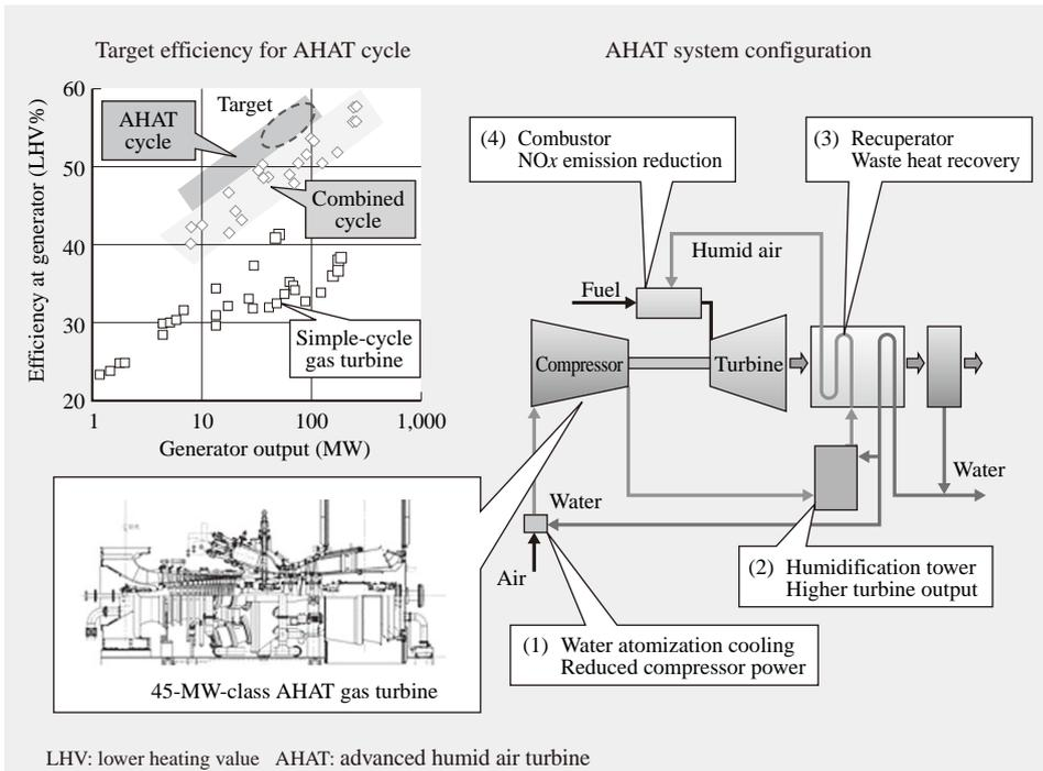
Fig. 9—AHAT System Configuration and Efficiency. The aim for the AHAT system is to achieve an efficiency equal to or better than that of a combined cycle plant despite using only a gas turbine.
