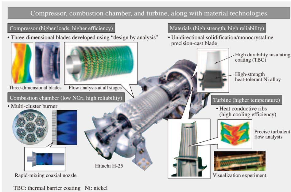
Fig. 7—Gas Turbine Research and Development Examples. To improve efficiency and reduce the environmental burden, Hitachi is working on a broad range of research and development covering the compressor, combustion chamber, and various material technologies, as well as the turbine unit itself.
