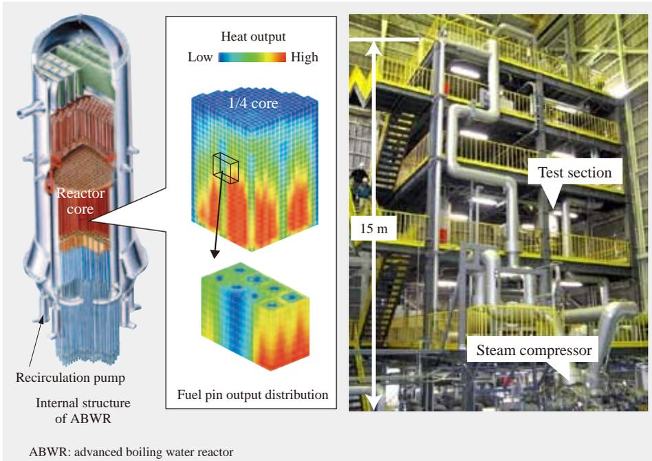
Fig. 11—Advanced Nuclear Reactor Simulation Techniques and a Demonstration Test Facility. Hitachi is utilizing methods, such as three-dimensional simulation of the core, to determine detailed thermal power distributions and conducting steam-water thermal-hydraulic testing at temperatures and pressures that occur in actual reactors to develop equipment with high performance and reliability.
