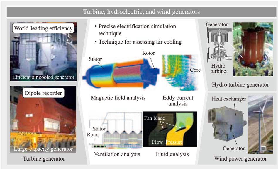
*Fig. 13—Generator Development. Hitachi is taking active steps to adopt simulation techniques as a way of ensuring the reliability of various types of generator, improving generation efficiency, and meeting the customer's requirement.*
