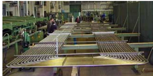
Fig. 13—Super Heater Panel Using Ni Alloy. HPE is undertaking a series of technical developments required for the building of 700°C-class boilers.
