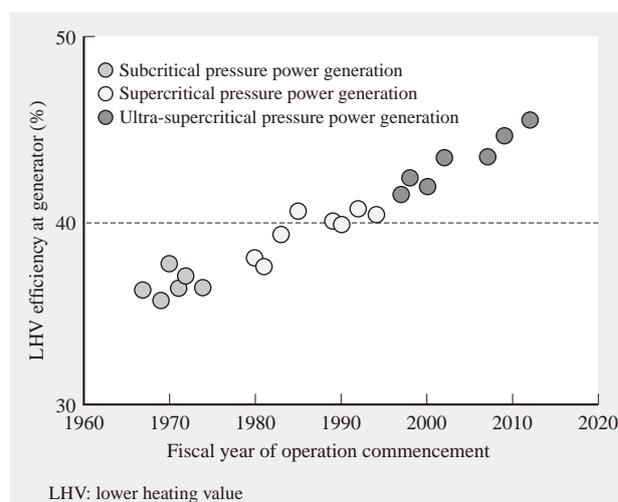
Fig. 1—Efficiency Improvement of Coal-fired Thermal Power Plants.
