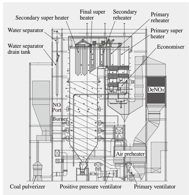
Fig. 6—Side Elevation Drawing of Torrealvaldliga Nord Boiler.
