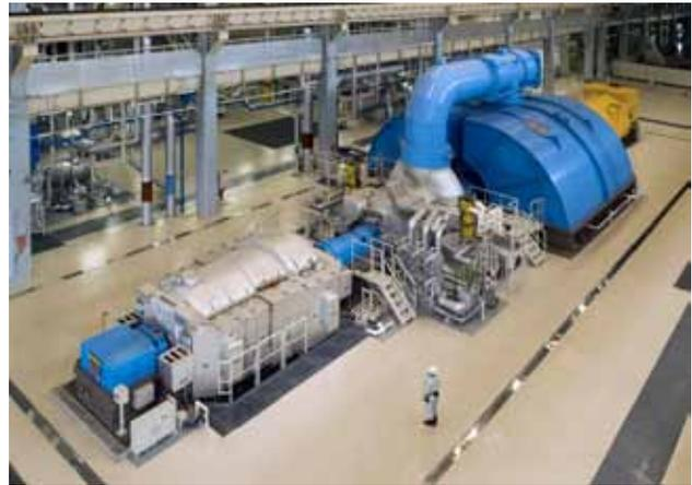
Fig. 3—New No. 2 Turbine Supplied to Isogo Thermal Power Plant of Electric Power Development Co., Ltd. The turbine operates with world-leading steam conditions, with a main steam pressure of 25 MPa, main steam temperature of 600°C, and reheat steam temperature of 620°C.
