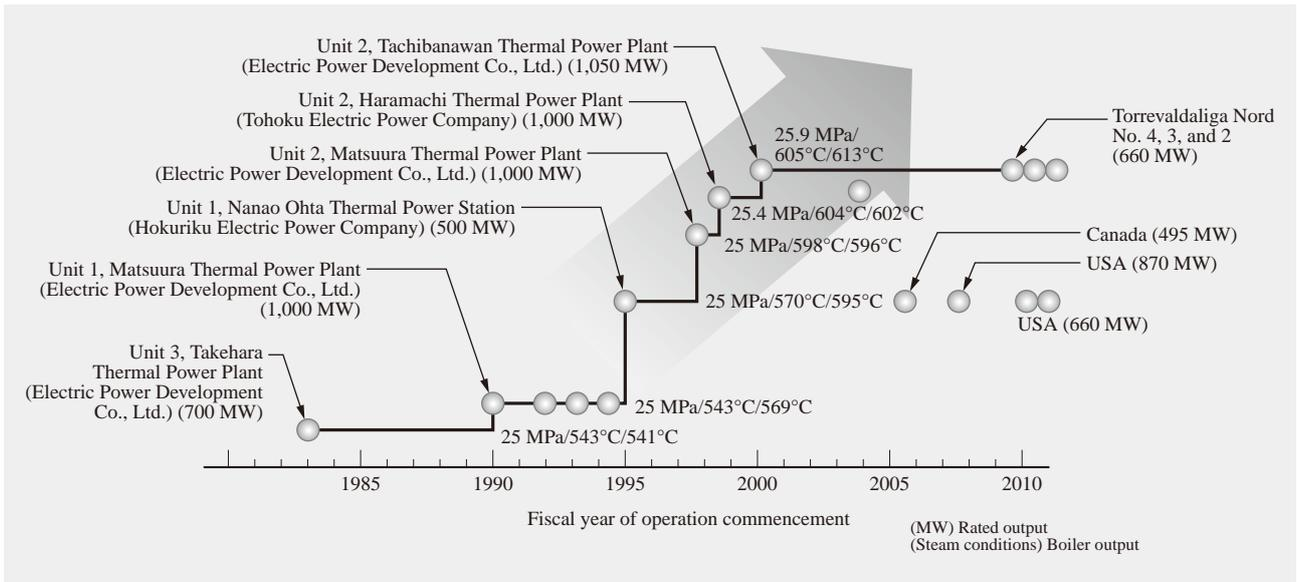
Fig. 4—Evolution of Steam Conditions of Plants Supplied by Babcock-Hitachi K.K.
