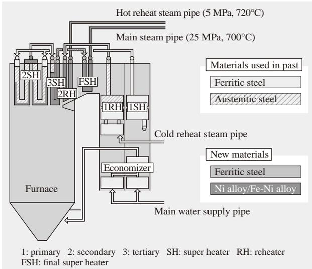
Fig. 10—Uses of A-USC Boiler Materials. Use of Ni alloy is limited to high-temperature parts.
