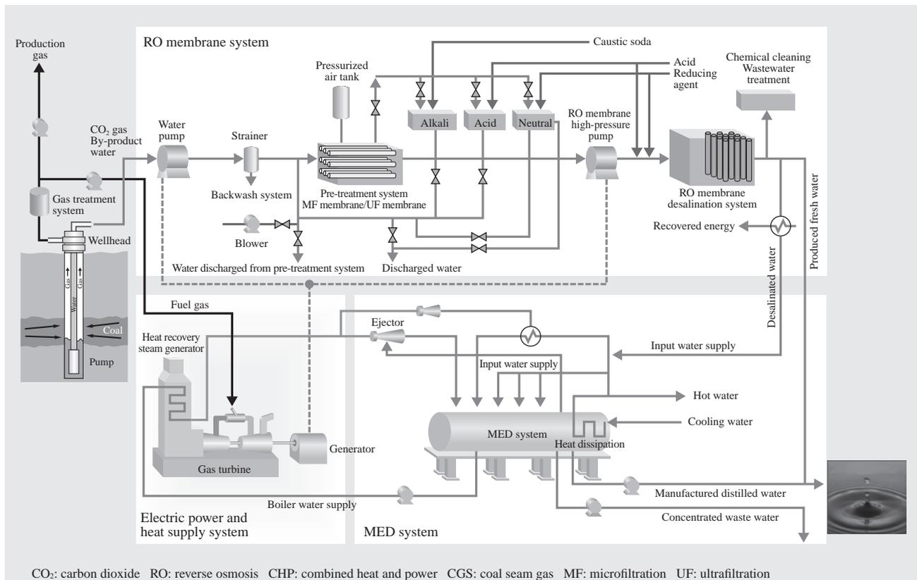
Fig. 4—Example Configuration of Hybrid Trigeneration System. Overview of a hybrid trigeneration system in which partially concentrated brine from an RO membrane system is further concentrated by an MED system that uses waste heat from a gas turbine.
