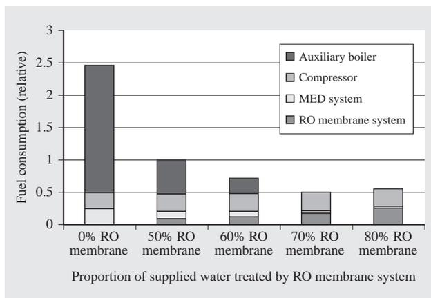
Fig. 5—Optimization of Hybrid System. The graph shows examples of the overall energy consumption calculated for different combinations of RO membrane and MED system operation.
