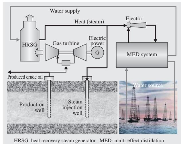
Fig. 3—Trigeneration System Producing Electric Power, Heat, and Water.
