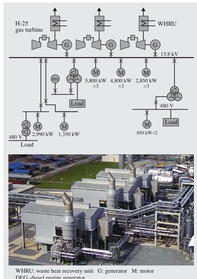
Fig. 1—Gas Turbine Cogeneration System.
