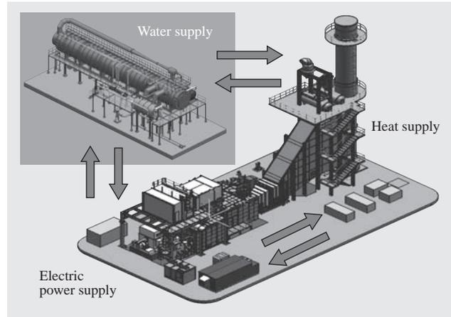
Fig. 6—Interrelation between Electric Power, Heat, and Water Supply in Trigeneration System.
