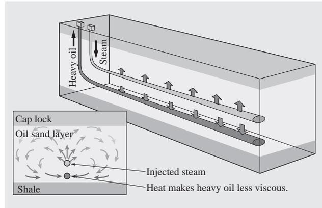
Fig. 2—Overview of SAGD Method for Heavy Oil Extraction. The diagram shows how the SAGD method extracts heavy oil.
