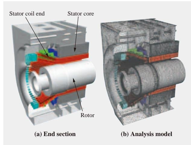
Fig. 7—Turbine Generator End Section and Analysis Model. The conjugate heat transfer analysis uses a three-dimensional loss distribution obtained by a magnetic field analysis to calculate both the ventilation characteristics and local temperatures.
