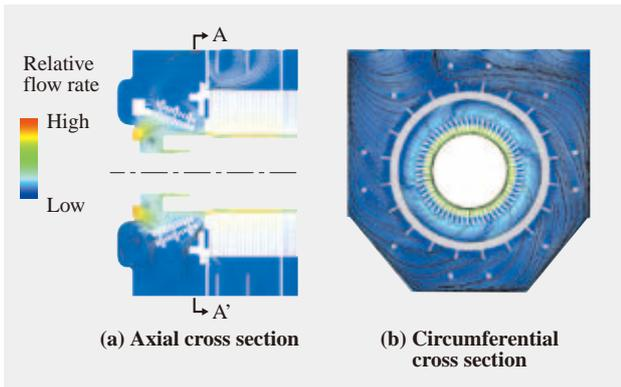
Fig. 8—Flow Rate and Streamline Distribution. This example shows a detailed analysis of the flow of coolant gas in a turbine generator. The A-A' arrows in the axial cross section (a) indicate the plane of the circumferential cross section (b).
