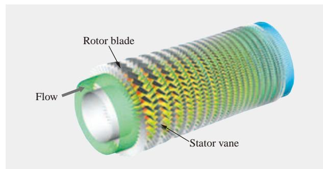
Fig. 5—Analysis of Multistage Axial Compressor.
