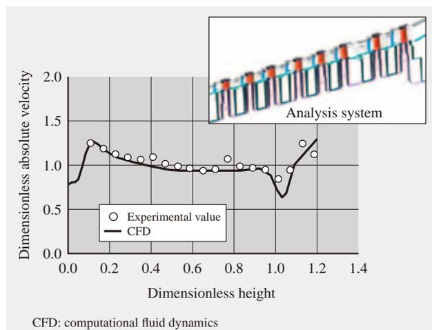
Fig. 2—Results of Three-dimensional Analysis of Multi-stage Steam Flow (CFD Analysis).
