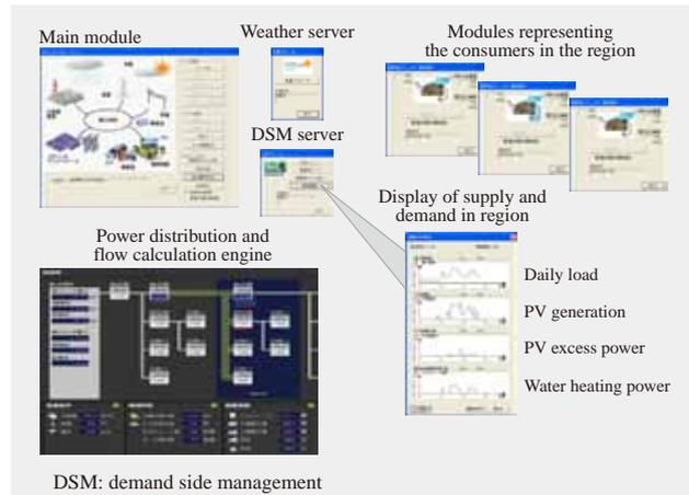
Fig. 11—Module Structure and Key Screens from Prototype System for Control of Local Photovoltaic Power Generation and Consumption.
