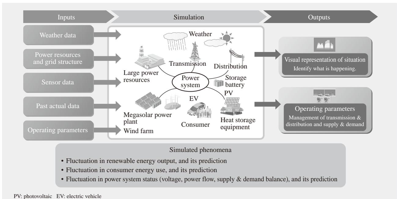
Fig. 10—Overview of Smart Grid Simulator.
