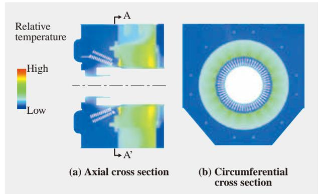
Fig. 9—Temperature Distribution. This example shows an analysis of the local temperatures in the coolant gas and structural components. The A-A' arrows in the axial cross section (a) indicate the plane of the circumferential cross section (b).
