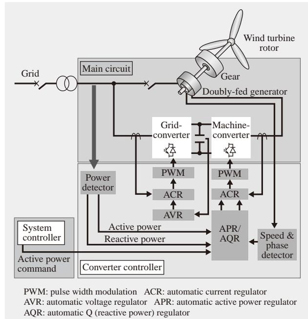
Fig. 5—Configuration of Power Conditioning System. The generator (rotor) current is controlled so that the system active power measured in the main circuit is kept equal to the active power command from the wind turbine controller.
