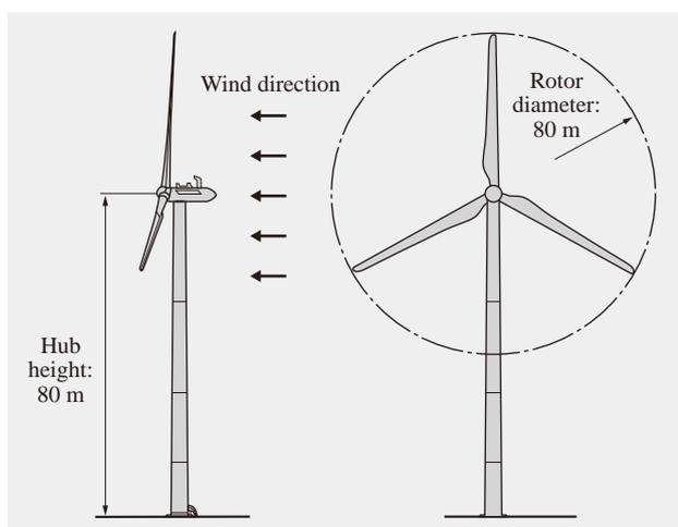
Fig. 1—Large Wind Turbine System.
