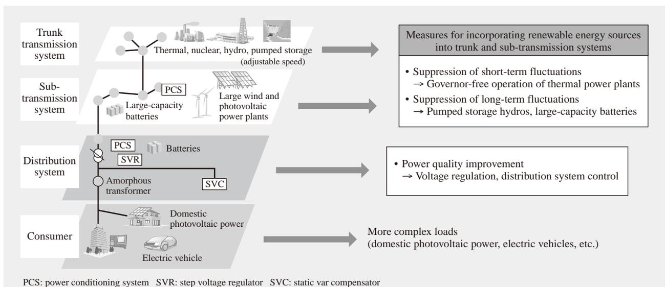
Fig. 8—Next-generation Power System (Smart Grid).
