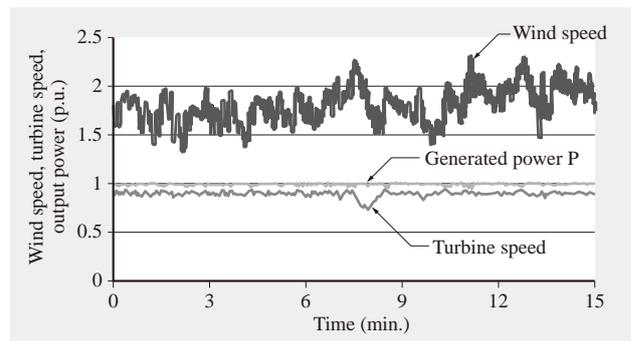
Fig. 6—Effect of Active-power-based Control. The system is able to draw down the energy in the rotating parts to keep the generated power (P) constant when there is a drop in wind speed.
