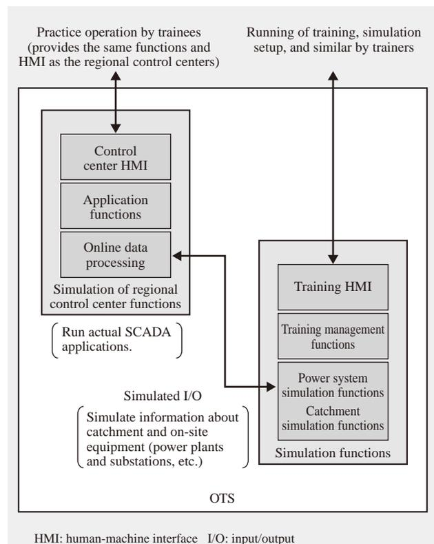
Fig. 2—Functional Configuration of OTS.
