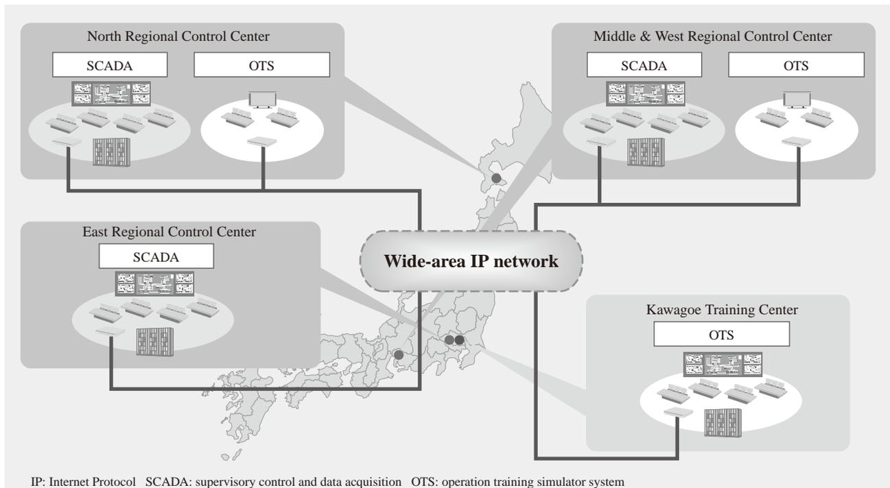
Fig. 1—Block Diagram of SCADA and OTS.
