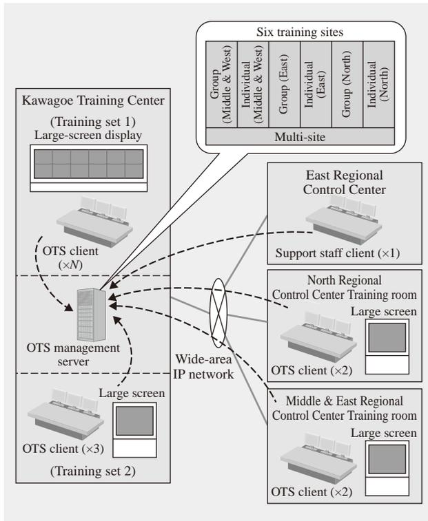
Fig. 3—Block Diagram of OTS.
