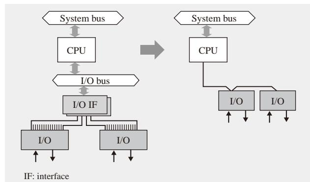
Fig. 4—Comparison of Old and New I/O Functions. Whereas the old I/O interface consisted of parallel signals from the CPU, new series of digital relays minimizes wiring by interfacing via a serial link from the CPU. This provides flexibility for adding extra I/O or other modifications.
