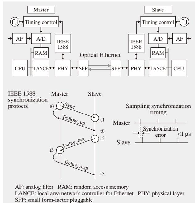
Fig. 3—Configuration of Sampling Synchronization Function Using IEEE 1588 Protocol. Slave devices exchange IEEE 1588 synchronization control packets with a master device to synchronize with their sampling timings. This system is implemented in hardware to achieve nanosecond-order precision.
