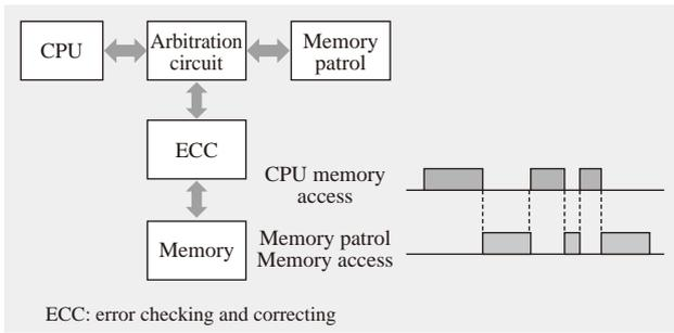
Fig. 5—Overview of Memory Patrol Function. The memory patrol circuit periodically uses the ECC circuits to check memory data integrity using times when the CPU is not accessing memory. It is able to correct single-bit errors.
