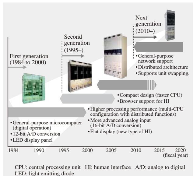
Fig. 1—Development Roadmap for Hitachi Digital Relays. Hitachi has developed a third generation of digital relays. The first generation was released in 1984.
