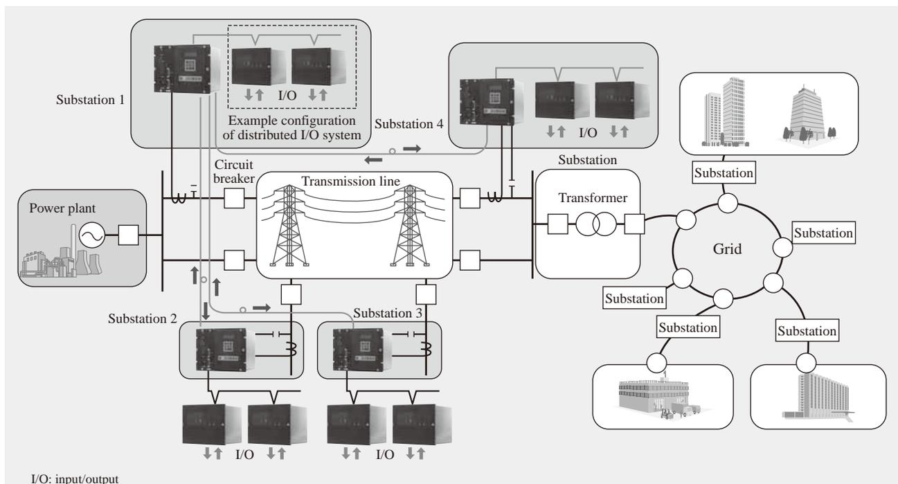
Fig. 2—Example Configuration of Distributed System Using New Digital Relays.
