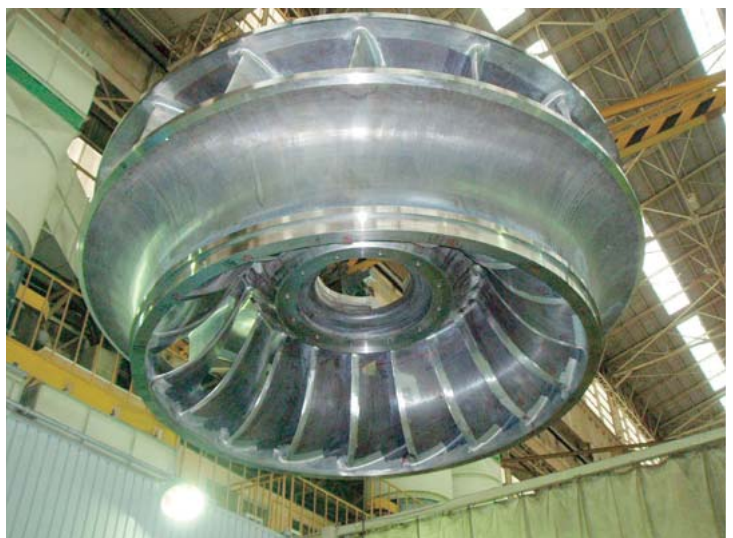
81.1-MW Francis turbine runner for Tangga Power Plant in Indonesia
