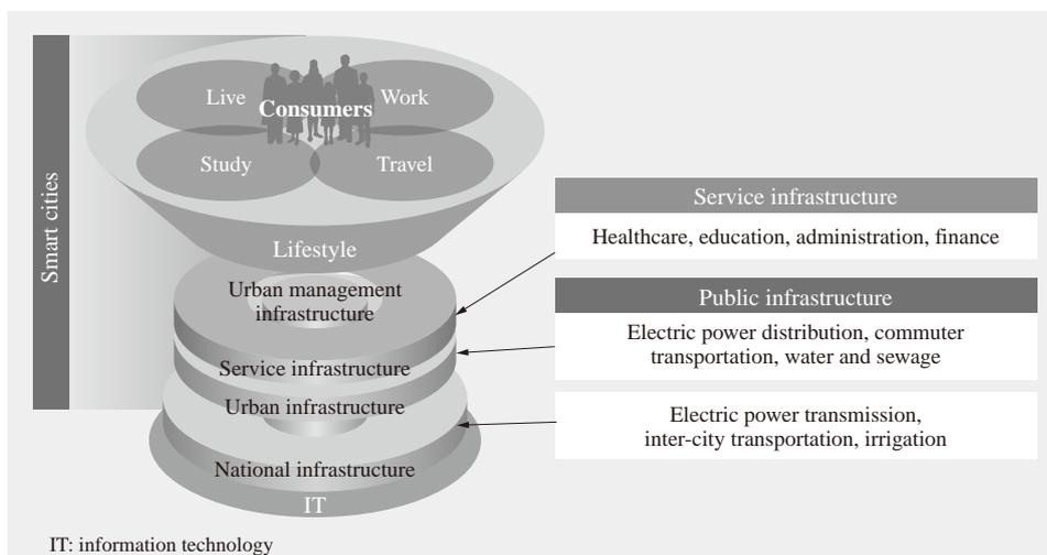
Fig. 2—Hierarchical Structure of Smart Cities. Smart cities consist of urban management infrastructure and two infrastructure layers for public services built on top of the national infrastructure.
