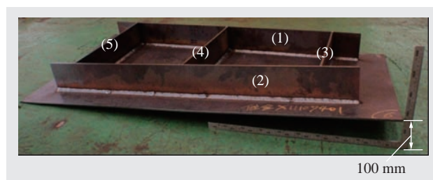
Fig. 4—Welding Structure Used for Experimental Testing.
