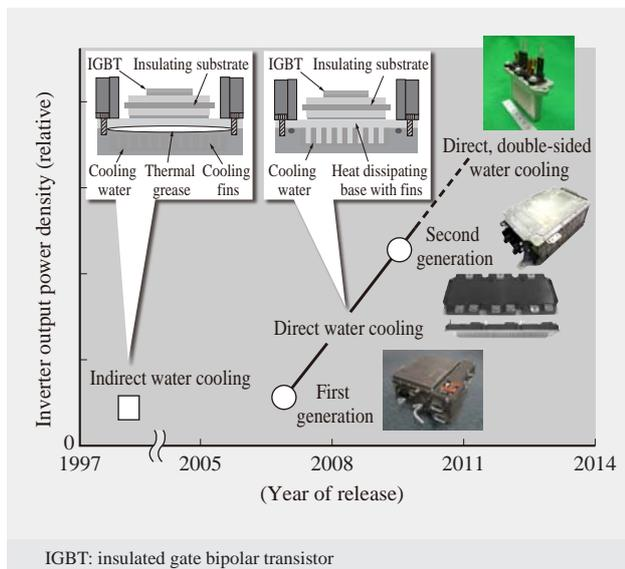
Fig. 2—Development Roadmap for HEV and EV Inverters. To satisfy the diverse requirements associated with use in a vehicle, Hitachi has developed direct water cooling to achieve smaller size and higher performance by utilizing implementation and analysis techniques derived from numerous other fields, such as the electric power, industrial, and consumer sectors.
