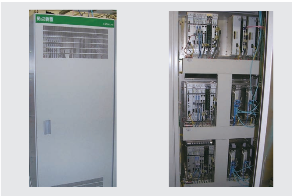
Fig. 8—Fail-safe Ground Unit for ATACS.
