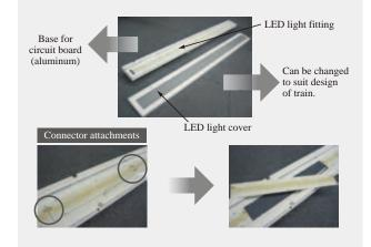
Fig. 3—LED Light Design and LED Circuit Board. The light fitting in which the circuit board is installed is made of aluminum and the cover is made of toughened glass over which is spread a highly transparent diffuser sheet. The LED circuit board is designed for easy replacement of individual blocks.
