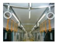
Fig. 6—Direct LED Lighting Installed in New Series 817 Trains Supplied to Kyushu Railway Company. These interior ceiling lights installed in a typical A-train provide a simple and expansive interior space.
