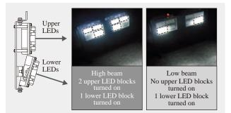
Fig. 8—High and Low Beam Operation. The high beam light uses the two upper blocks and one lower block. The low beam light uses one lower block. If one block fails, the system can switch on an adjacent block as a replacement.
