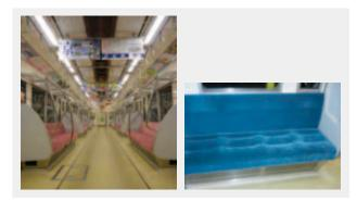
Fig. 2—Train Interior Using LED Lighting with Strong Yellow Component and Blue Seat.
