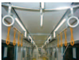
Fig. 6—Direct LED Lighting Installed in New Series 817 Trains Supplied to Kyushu Railway Company.
