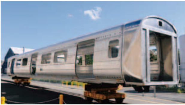
Fig. 8—Carbody. The carbody has a lightweight aluminum structure that complies with CR-TSI.
