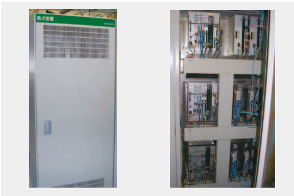
Fig. 8—Fail-safe Ground Unit for ATACS.
