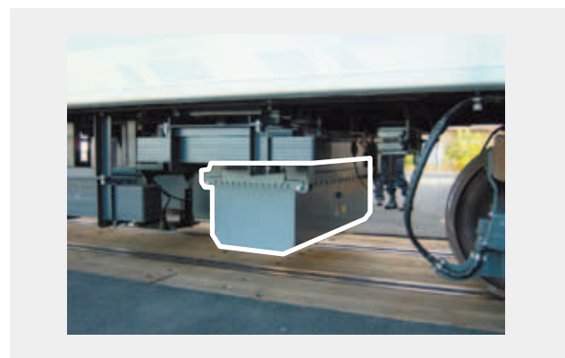
Fig. 9—Inertial Mid-chord Offset Track Measurement System for Mounting on Carbody.
