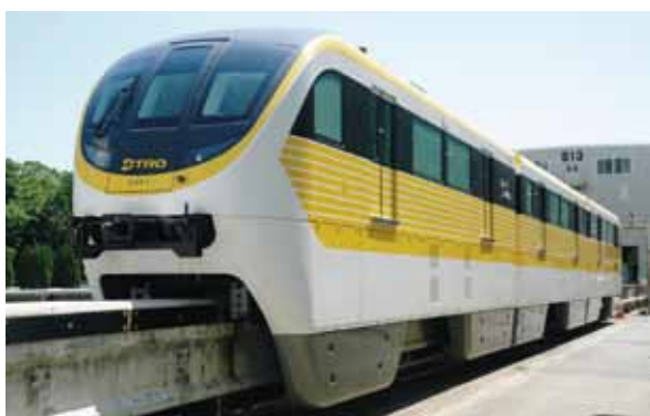
Monorail car for Line 3 of the Daegu Metropolitan Transit featuring latest unattended operation and safety equipment.
