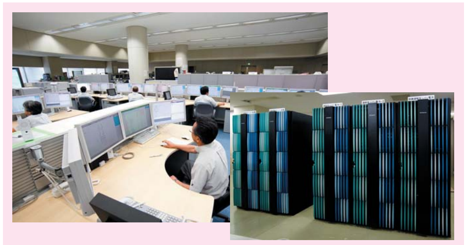
Power system supervision using East Japan Railway Company's train supervisory control and data acquisition system for the Tokyo metropolitan area (control sub-system) and blade servers designed for control applications
