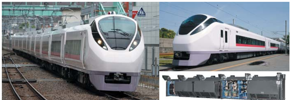
East Japan Railway Company Series E657 AC/DC express train in commercial operation (left), prior to delivery from Kasado Works (top right), and the main converter/inverter transformer system (bottom right)
