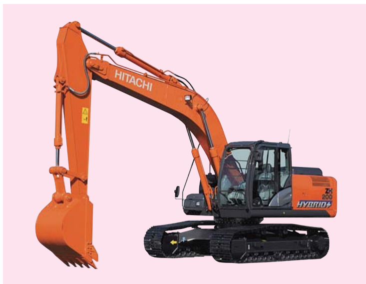
ZH200 hybrid hydraulic excavator (operating mass: 20,100 kg)
