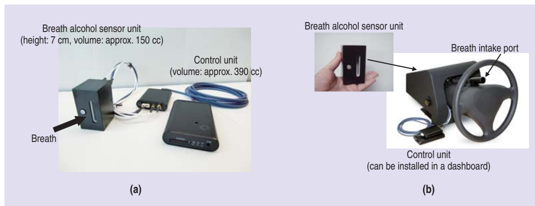
Prototype breath alcohol detection system (a) and steering wheel installation example (b)
