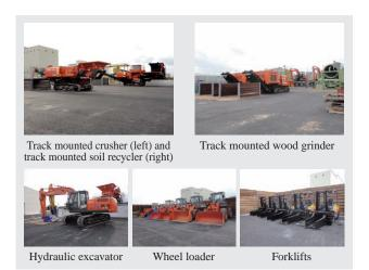
Fig. 2—Tagajo City Project for Interim Disposal of Rubble and Other Waste Material from the Great East Japan Earthquake. The work utilizes all types of recycling machinery, such as track mounted wood grinders and track mounted screens, as well as hydraulic excavators, wheel loaders, and also forklifts made by TCM Corporation, a subsidiary of Hitachi Construction Machinery Co., Ltd.
