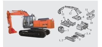
Fig. 9—1.0-m<sup>3</sup>-class Disassemblable Hydraulic Excavator in Assembled and Disassembled Forms (Excluding Accessories). The design includes use of flanges on detachable parts of structural components, one-touch hydraulic couplings, electrical connectors, and a weight that can be split into upper and lower halves.
