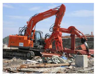
Fig. 5—Rubble Clearance (at Minamisanriku-cho). The main arm holds up steel framing and pulls it away from building foundations so that the cutter attached to the auxiliary arm can cut it free.
