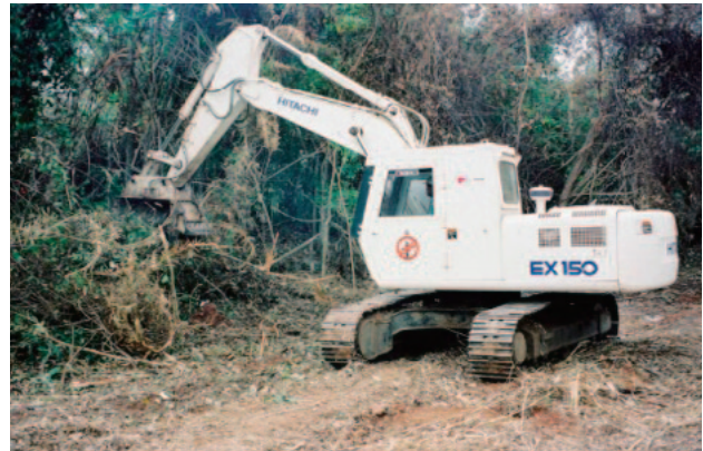
Fig. 2—Swing Type Anti-personnel Landmine Removal Machine Able to Deal with Brush Efficiently Using Rotary Cutter.
