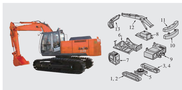
Fig. 9—1.0-m 3 -class Disassemblable Hydraulic Excavator in Assembled and Disassembled Forms (Excluding Accessories). The design includes use of flanges on detachable parts of structural components, one-touch hydraulic couplings, electrical connectors, and a weight that can be split into upper and lower halves.
