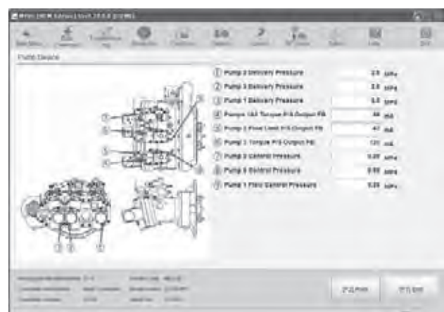
Fig. 9—Example Screen on Fault Diagnostics System. The example screen from the fault diagnostics system shows the main pump pressure.
