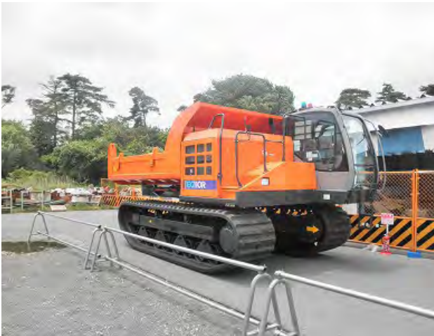
Fig. 6—Radio-controlled Crawler Carrier. This EG110R crawler carrier was modified for radio control and supplied to the site together with the remote controller (specified low-power 429-MHz band).
