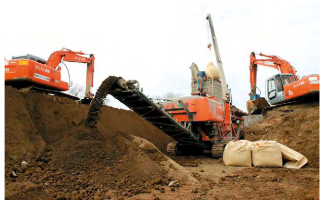
Fig. 3—Track Mounted Soil Recycler and Other Construction Machinery Used for Civil Engineering Reconstruction Work. It is anticipated that the track mounted soil recycler and other machines will be used for tasks such as stabilization of soft ground, roadbed construction, and repairing of washed-away riverside embankments.
