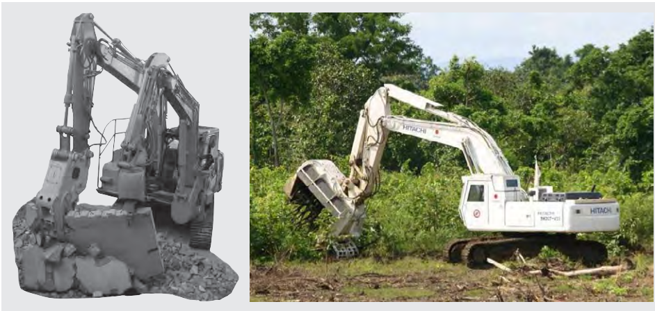
Fig. 8—Double-arm Working Machine (Left) and Demining Machine (Right). Machines such as the double-arm working machine and demining machines help with disaster recovery and with restoring the land to peace and prosperity.
