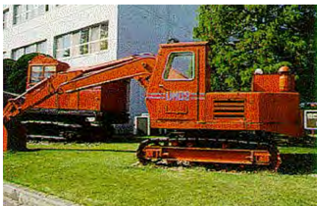
Fig. 3—First Hydraulic Excavator Based Entirely on Japanese Technology (UH03).
