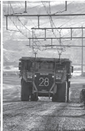
Fig. 6—Trolley-assisted Dump Truck Incorporating Technology from Hitachi Group. This trolley-assisted dump truck was developed using technology from across the Hitachi Group and is being sold as a package that includes the overhead contact lines.
