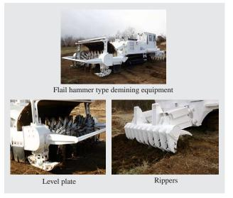
Fig. 3—Flail Hammer Type Demining Equipment. After landmines are cleared by the highly explosion-resistant flail hammer fitted to the front of the machine, the soil is plowed by rippers fitted to the rear to help restore it to agricultural use.
