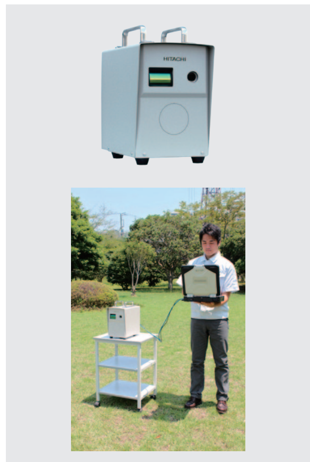
Fig. 1—External Appearance of Gamma Camera Radiation Measurement Device and Example of Usage.
