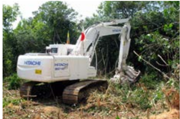
Fig. 1—Swing Type Anti-personnel Landmine Removal Machine Able to Deal with Brush Efficiently Using Rotary Cutter. The rotary cutter is used to clear the brush to make the landmines easier to find. The unit can swing backwards and forwards to follow the lie of the land and perform clearance work even on sloped or other uneven terrain.
