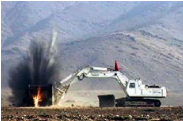
Fig. 2—Explosion Resistance Testing in the Islamic Republic of Afghanistan.
