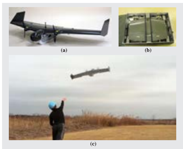
Fig. 6—Exterior of UAV (Short-distance) JUXS-S1 and Thrown Takeoff.
