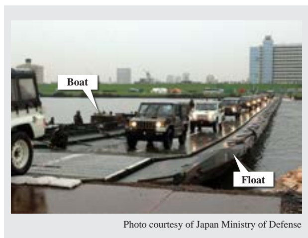
Fig. 1—Bridge Construction and Vehicles Driving over Type 92 Floating Bridge.
