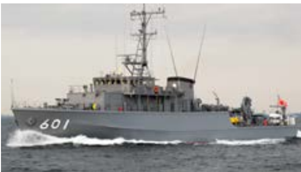
Fig. 2—Minesweepers Equipped with Mine Hunting Sonars. A minesweeper guards the safety of the ocean by removing mines laid underwater and on the seafloor.
