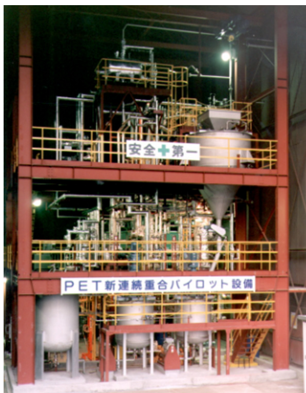
Fig. 4—Pilot Plant at Hitachi. The pilot plant can be used to test continuous processes.
