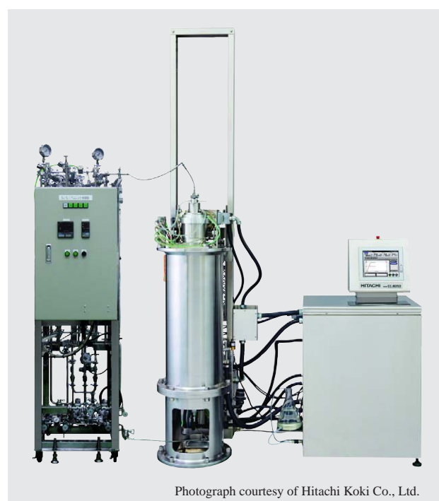
Fig. 2—Ultracentrifuge Used for Virus Separation. This ultracentrifuge for virus separation made by Hitachi Koki Co., Ltd. operates at approximately 110,000 G to separate viruses from the recovered fluid.
