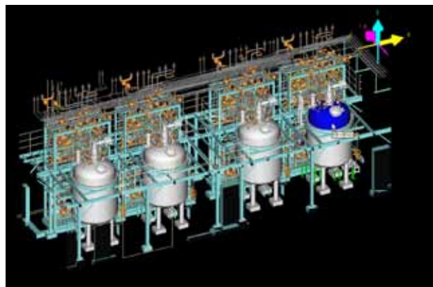
Fig. 3—Three-dimensional Computer-aided Design Image of Tank and Pipe Module.
