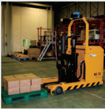
Fig. 2—Main Specifications of Autonomous Forklift AGV. Witness test was conducted using dummy loads.
