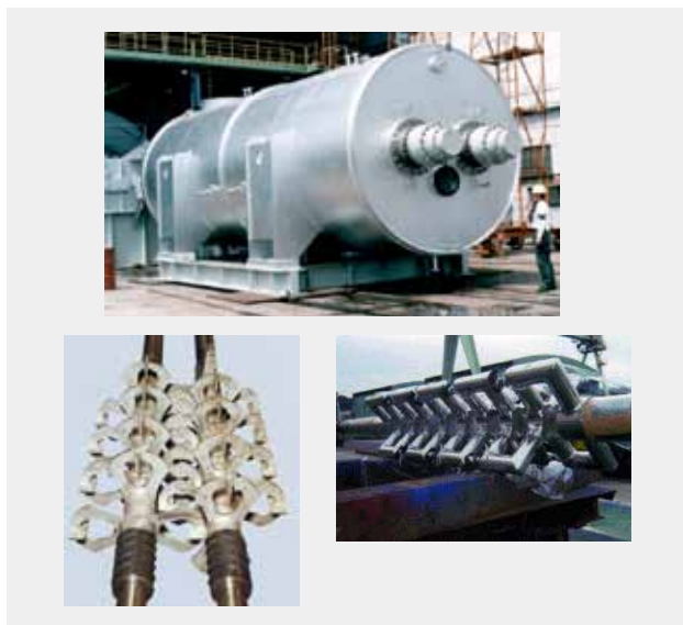
Fig. 6—High-viscous Material Processing Technology. The polycondensation reaction in the bioplastics production process requires agitation to be performed to remove byproduct gas from the highly viscous molten polymer. Hitachi has extensive know-how in the design of the reaction tank and agitators required to achieve this.
