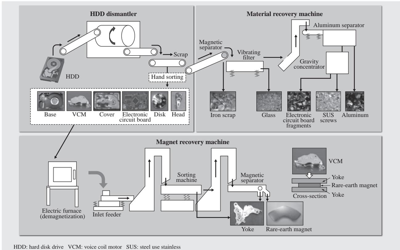
Fig. 2—Process Used to Separate and Recover Rare-earth Magnets from HDDs. Hitachi has developed and commercialized a process that separates the rare-earth magnets from HDDs and also sorts the other scrap to automatically separates fragments of precious metals or other valuables.
