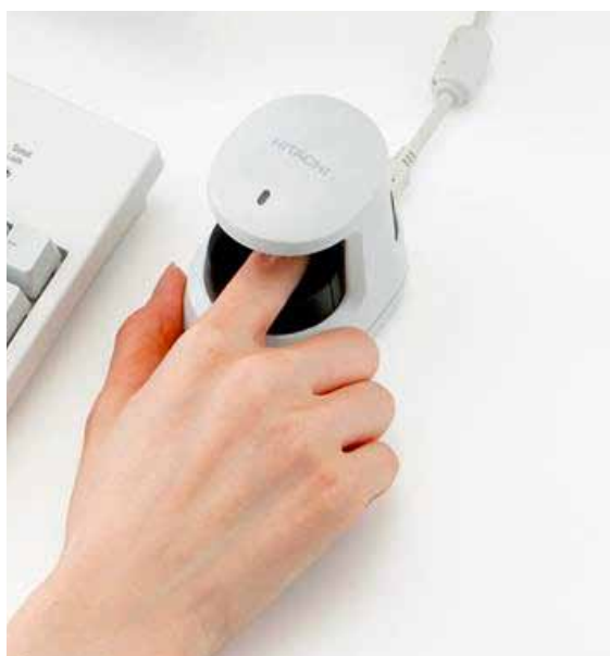
Hitachi finger vein authentication system. The system is used for personal identification at bank ATMs.
