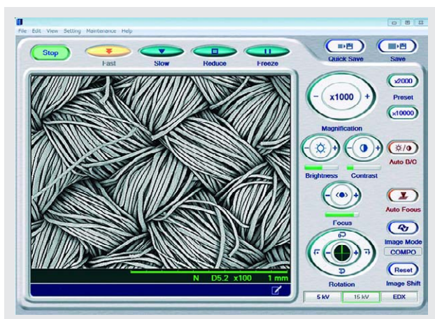
Fig. 3—Screen Shot from TM3000 Tablet Microscope. The screens are designed to be intuitive and easy to understand, and a full range of automatic functions that can perform adjustments at a single touch makes operation easy and magnification changes smooth.
