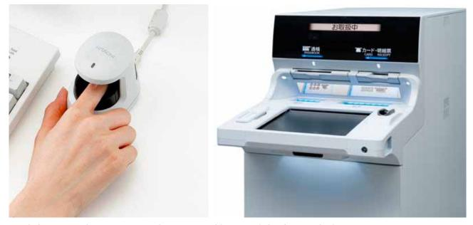
Hitachi finger vein authentication system. The system is used for personal identification at bank ATMs.
