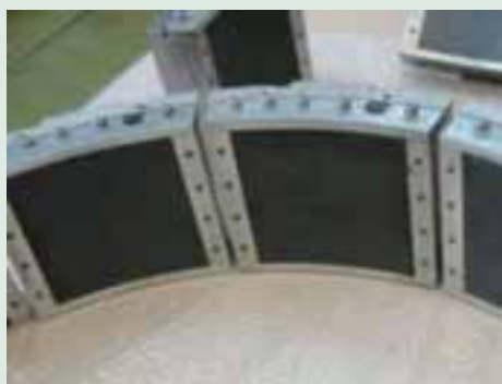
Water-lubricated resin bearing in Kaplan turbine (left) and black PPS bearing pads (right)
