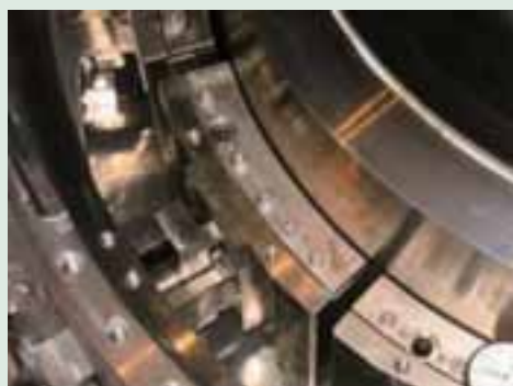
Water-lubricated resin bearing in Kaplan turbine (left) and black PPS bearing pads (right)
