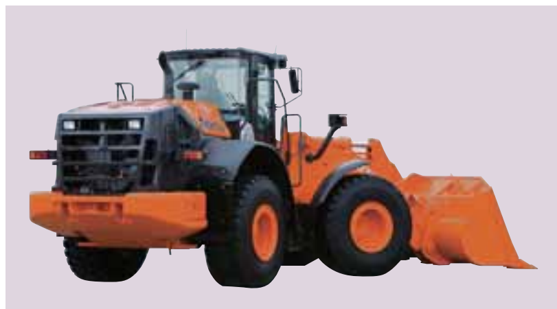
ZW250-5B wheel loader compliant with European Stage IIIB exhaust emission standards
