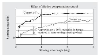
Fig. 10—Effectiveness of Friction Compensation Control. A control system that compensates for friction in mechanical systems provides a smoother feel to the steering by significantly reducing the torque required to start turning the steering wheel from the center position.
