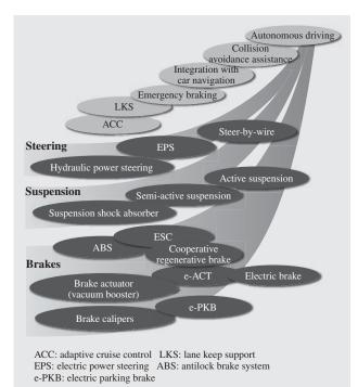
Fig. 2—Advances in Chassis Control Systems.
