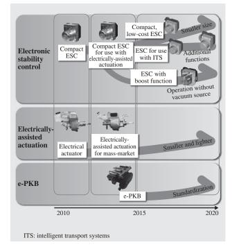
Fig. 3—Roadmap for Controlled Brakes. With a product range that includes skidding prevention systems, electric actuator, and e-PKBs, Hitachi supplies brake systems that cover everything from normal driving conditions to extreme cases.
