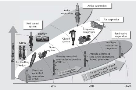
KDSS: kinetic dynamic suspension system HBMC: hydraulic body motion control \*HMBC is a product name of Nissan Motor Co., Ltd.
