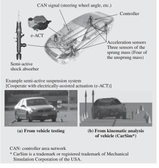
Fig. 6—Cooperative Control System for Semi-active Suspension and Controlled Brake.
