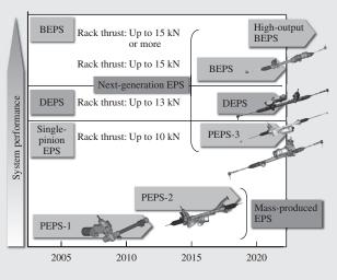
PEPS: pinion EPS DEPS: dual-pinion EPS BEPS: belt-drive EPS
