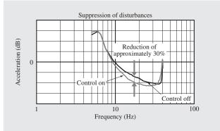
*Fig.* 9—*Effectiveness of Control Technique for Suppressing Disturbances.*
