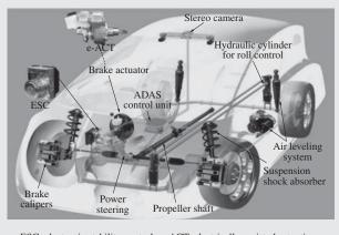
ESC: electronic stability control e-ACT: electrically-assisted actuation ADAS: advanced driver assistance system
