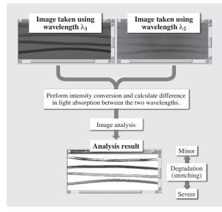
*Fig.* 5—Use of Dual-wavelength Optical Technique to Assess Cable Degradation.
