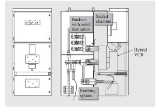
*Fig. 14—Panel with Solid Busbar Insulation for Overseas Markets.*
