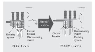
*Fig. 15—Advances in Vacuum-insulated Switchgear. Hitachi is developing the C-VIS+ to have an even simpler design than the C-VIS.*
