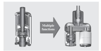
Fig. 2—Combination of Multiple Functions in Vacuum Interrupter. Switchgear is made smaller and lighter by using vacuum interrupters for both circuit breaker and disconnecting switch functions, rather than as single-function devices as in the past.
