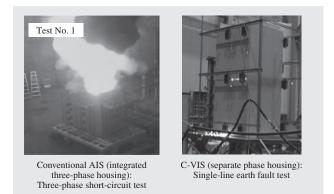
Fig. 11—Internal Arc Testing of Switchgear. Use of a design in which the phases are kept separate significantly reduced the consequences of internal arc accidents.
