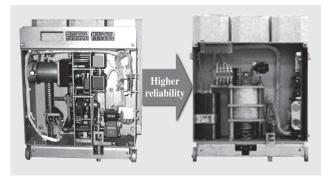
Fig. 1—Advances in VCB Operating Mechanisms. To improve the reliability of the mechanisms used to operate vacuum circuit breakers (VCBs), the spring mechanisms used in the past, which had many mechanical parts, have been replaced with hybrid electromagnetic mechanisms that have few parts.
