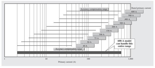
Fig. 13—Comparison of Current Compensation Ranges for Wide-range CT and Previous CT. The wide-range CT has a wide performance compensation range, reducing the need to replace the CT to handle higher loads.
