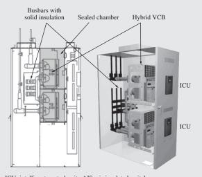
ICU: intelligent control unit AIS: air-insulated switchgear
