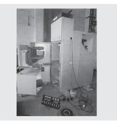
Fig. 7—Certification Testing of 12-kV Hybrid VCB for the Chinese Market.
