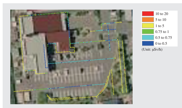
Fig. 4—Measurement of Dose Equivalent Rate Using PSF system. The data measured by the PSF system is displayed on a digital map to provide an accurate indication of the contaminated areas and to facilitate efficient and effective decontamination.
