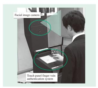
Fig. 2—Touch Panel Finger Vein Authentication System.
