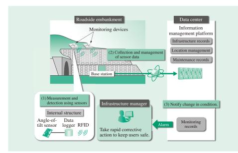
Fig. 3—Example of Condition Monitoring Service. This example is for a roadside embankment. The condition monitoring service monitors for situations such as landslides and issues realtime alarms.
