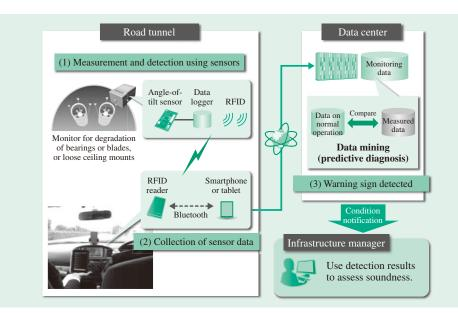
Fig. 4—Example of Predictive Diagnosis Service. In this example, a vehicle makes routine visits to collect sensor measurements. The predictive diagnosis service uses data mining techniques developed by Hitachi to detect warning signs of aging or other deterioration.
