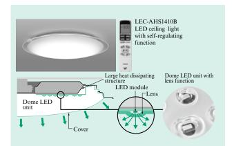
Fig. 3—Appearance and Technical Features of LED Ceiling Light. The figure shows a large heat dissipating structure and a dome LED unit with a lens function.
