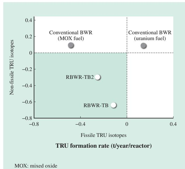
Fig. 9—Rate of Formation and Consumption of TRUs. A negative value indicates that consumption of TRUs results in a reduction in their quantity. The value for conventional BWRs is from Ando and Takano<sup>(8)</sup>.
