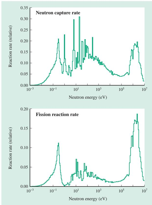
Fig. 10—Dependence on Neutron Energy of Neutron Capture and Fission Reactions in RBWR-TB Core.
