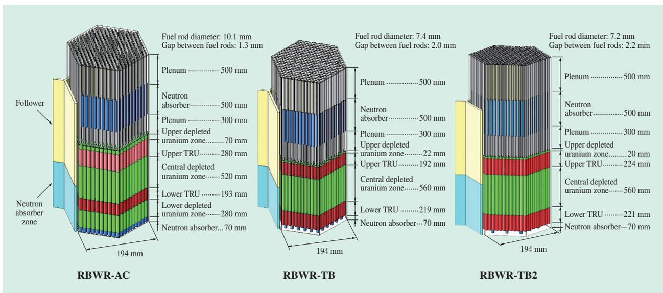
Fig. 7—RBWR Fuel Assembly. The height of the TRU and depleted uranium zones, the fuel rod diameter, and the gap between fuel rods are adjusted to ensure that the multi-recycling of TRUs can be performed in a way that suits the purpose of each reactor design. As the RBWR-TB and -TB2 TRU burner reactors have less need for TRU formation, their fuel assemblies do not include the lower depleted uranium zone.
