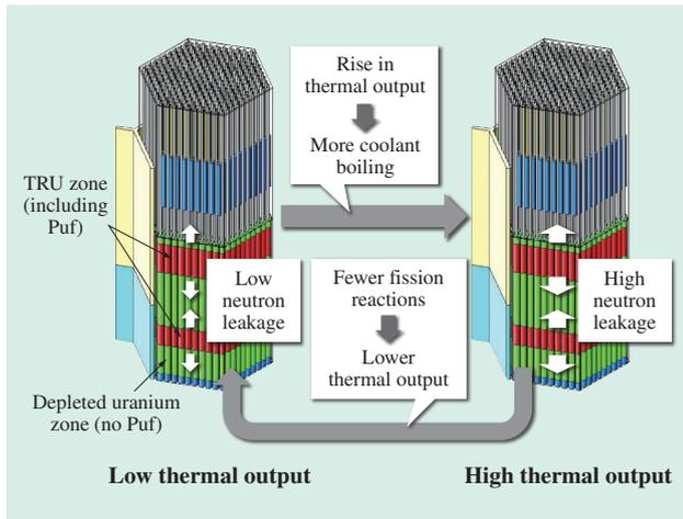
Fig. 2—Inherent Safety of RBWR.
