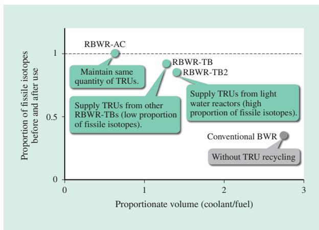
Fig. 8—Proportionate Volume of Coolant in RBWR and Conventional BWR Reactors.
