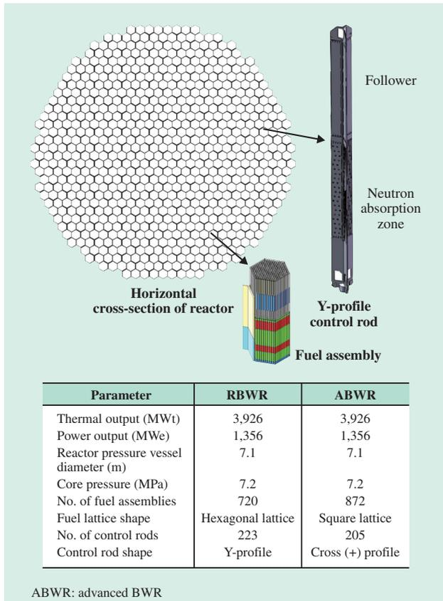
Fig. 6—Basic Specifications of RBWR Plant. The rated thermal output, power output, reactor pressure vessel diameter, and core pressure of the RBWR are the same as an ABWR. A follower is fitted to the top of each control rod to prevent water entering the space vacated when the control rod is withdrawn.
