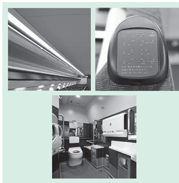
Fig. 3—Interior Fittings on Latest High-speed Shinkansen Rolling Stock. The internal fittings use the latest technologies such as LED lighting and are designed for barrier-free accessibility.
