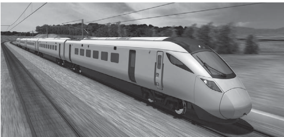
Fig. 6—Class 800/801 High-speed Rolling Stock for UK IEP. The rolling stock was developed by applying technologies developed in Japan for lighter weight and higher speed to UK railway systems.
