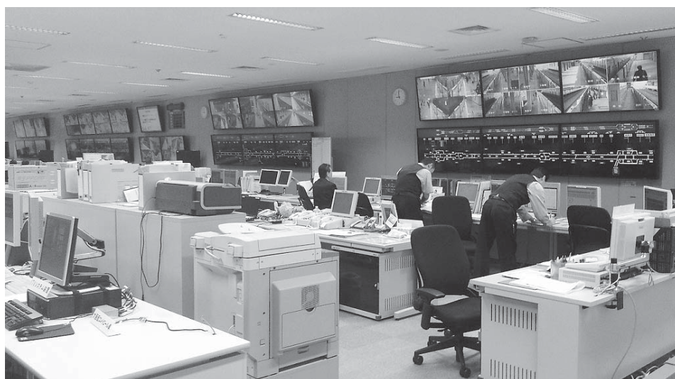
Fig. 7—Control Room at Integrated Control Center. Traffic monitoring and automatic control of all trains on four lines is handled from supervisory control desks and the traffic display panels for each line that are installed side-by-side in the control room.
