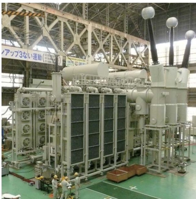
7 Factory testing of first 900-MVA-class power plant transformer (four transformers are to be supplied in total)
