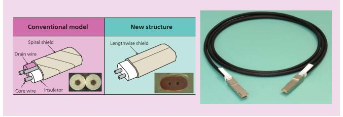
2 New structure for high-speed (25 Gbit/s) metal transmission cable (left) and harness using new structure cable (right)
