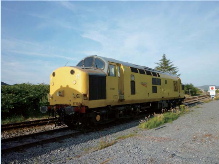
1 Class 97 locomotives fitted with Hitachi's on-board ETCS signalling system
