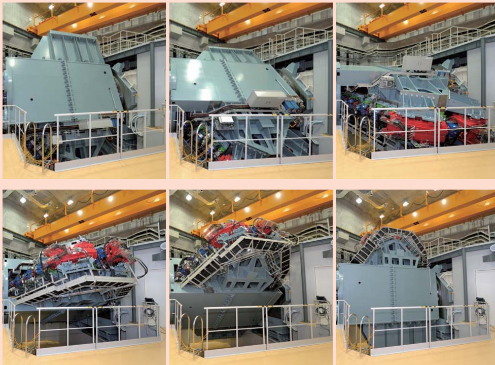
View from the rear of the treatment room as the gantry rotates. A comprehensive review of the design succeeded in downsizing the unit.
