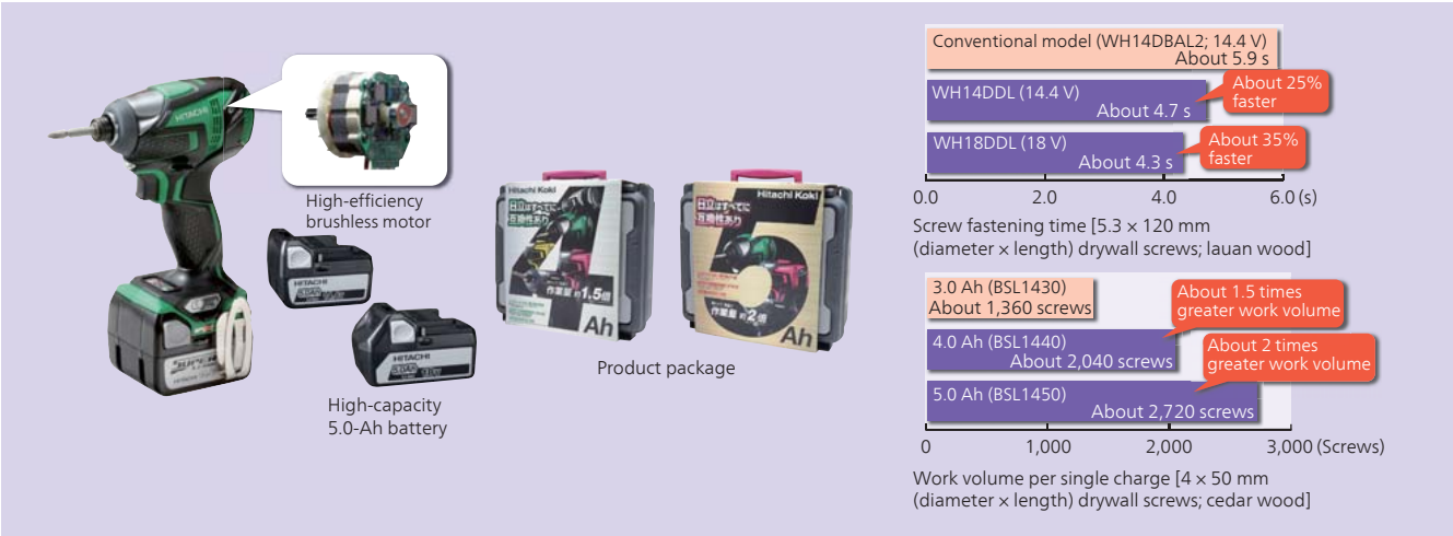
3 WH14DDL cordless impact driver (left) and comparison of screw fastening speed and work volume (right)
