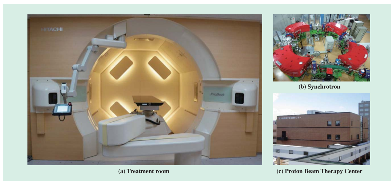
Fig. 1—Proton Beam Therapy System at Hokkaido University Hospital Proton Beam Therapy Center. (a) Treatment room equipped with rotating gantry. The irradiation field shaping mechanism (located under the table) enables the proton beam to be directed at the patient from any angle (360°). (b) The proton beam is accelerated by a synchrotron accelerator. (c) The Proton Beam Therapy Center is located next to Hokkaido University Hospital for easy access by patients.
