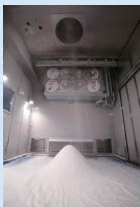
7 Test room when the solar simulator lights are on (top) and test room after continuous operation of the snow simulator (bottom)
