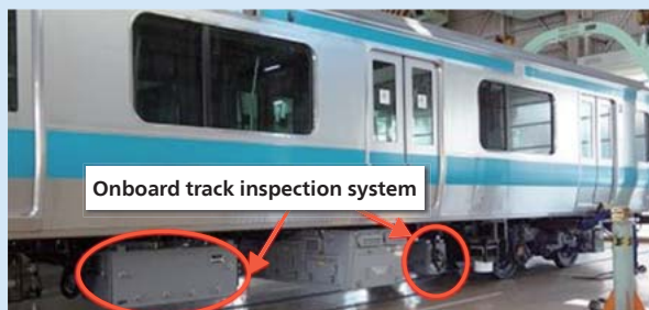
7 East Japan Railway Company's onboard track inspection system
