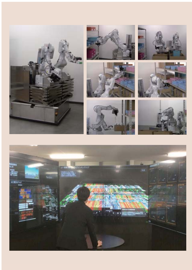
13 Operation of autonomous mobile dual-arm robot (top) and cockpit (bottom)
