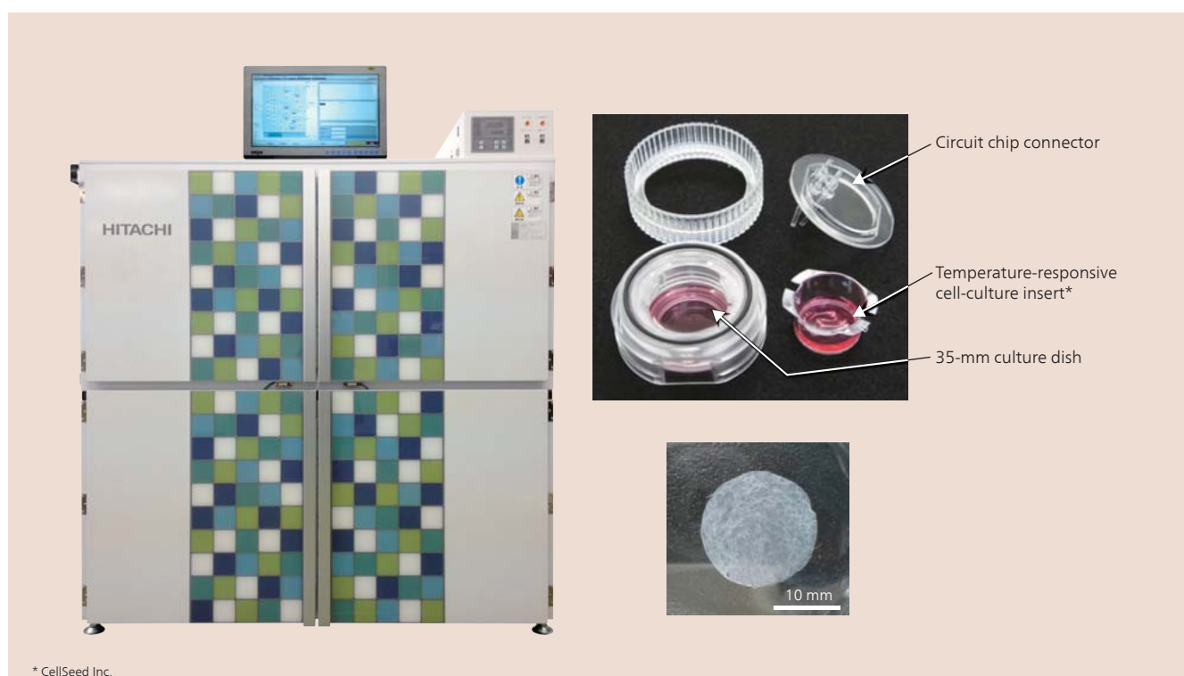
5 ACE3 automated cell culture system (left), closed culture vessel (top right), and cell sheet after automatic culture in an ACE3 (bottom right)
